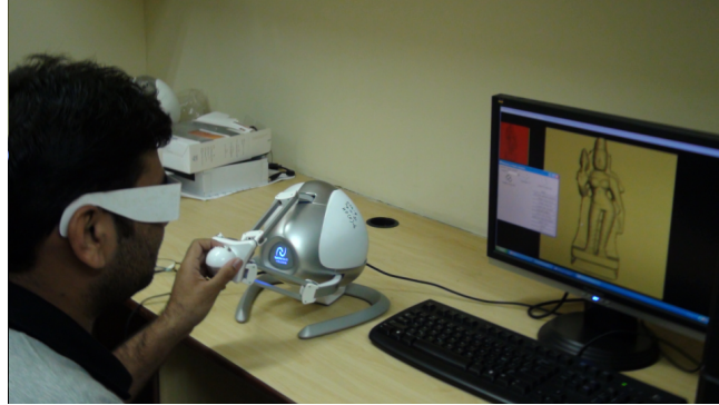
Fig. 11. Illustration of hpto-visual immersion of a subject for a 3-D object. On the left, the user wearing anaglyphic glasses is holding the FALCON haptic device while interacting with the virtual 3-D object displayed on the screen.
